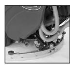
For a full functioning scrubber, move the hose to the squeegee and lower the squeegee to the floor.
